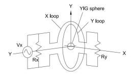
Figure 2: Magnetic resonance filtering
