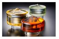
communication devices such as resonators, filters, transducers, etc., especially for the manufacture of high-frequency surface acoustic wave devices due to their good electromechanical coupling, temperature coefficient and other comprehensive properties, and are used in Mobile phones, walkie-talkies, satellite communications, aerospace and many other high-end communication fields.
