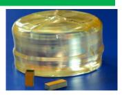
transduction material, ferroelectric material, electro-optic material, as an electro-optic material, it plays an optical modulation role in optical communication, and is widely used in parametric oscillators, frequency doubling, acousto-optic devices, and optical modulation device. The incorporation of MgO can effectively improve the anti-damage threshold of the crystal.
